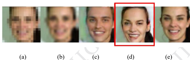
Figure 5. Output results of Class-info SRGAN by adding gender classifier ((a) 16×16 down-sampling; (b) bicubic interpolation; (c) SRGAN; (d) proposed; (e) 64×64 original)
